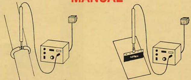
On pipe in-plant or in-yard, with spring electrode
